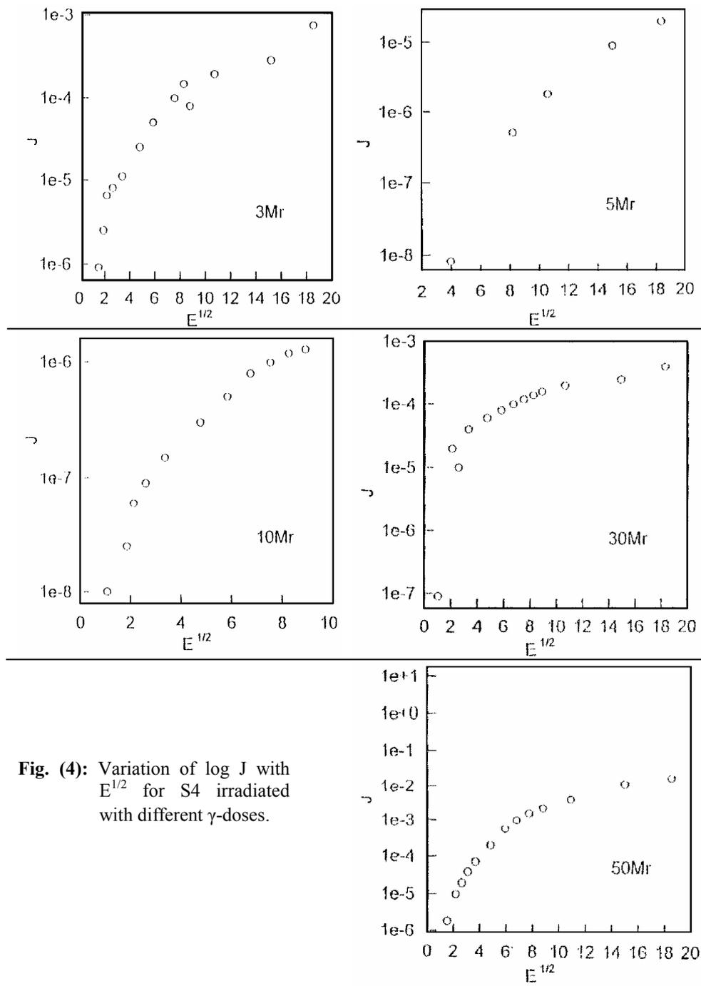
**Fig. (4):** Variation of  $\log J$  with  $E^{1/2}$  for S4 irradiated with different  $\gamma$ -doses.
