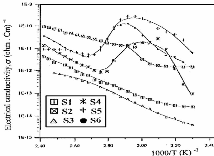
Fig. (1): The temperature dependence of the d.c. electrical conductivity for SBR samples loaded with different metallic filler (Fe/Cu) ratios.
