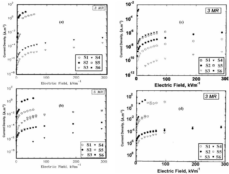
Fig. (2a-e): The current density-electric field characteristics for all samples irradiated with different  $\gamma$ -doses
