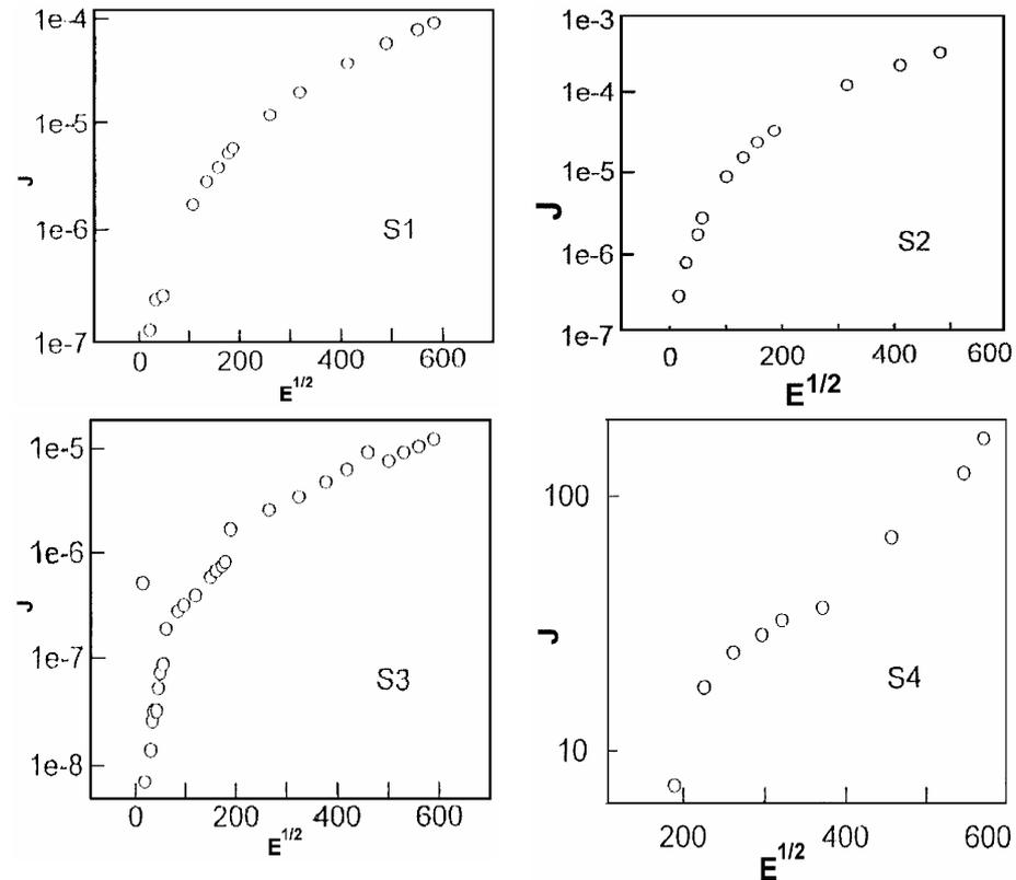
Fig. (3): Variation of log J with the square root of the electric field for all samples.
