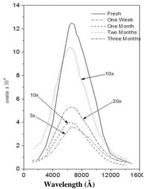
**Fig. (7):** Effect of aging on PL for samples immersed in ethanol for 40hr then passively etched for 3hr and aged up to 3 months.
