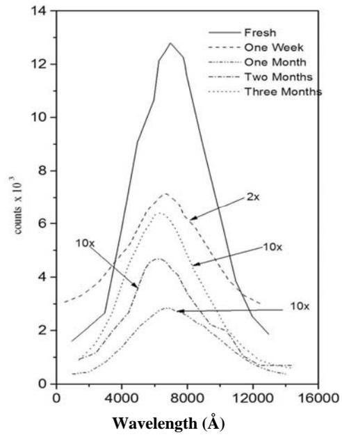
**Fig. (6):** Effect of aging on PL for samples immersed in ethanol for 20hr then passively etched for 4hr and aged up to 3 months.
