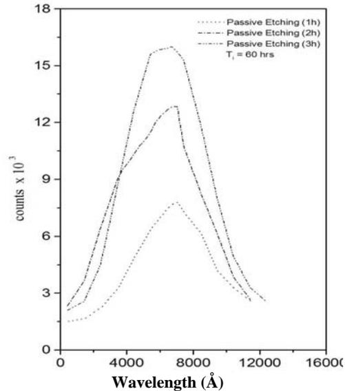
**Fig. (4):** PL spectra of freshly prepared PSLs and after immersion in ethanol for 60hr then passively etched
