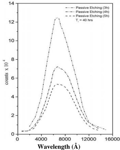
**Fig. (3):** PL spectra of freshly prepared PSLs and after immersion in ethanol for 40hr then passively etched
