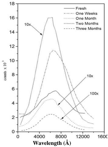
**Fig. (5):** Effect of aging on PL for samples immersed in ethanol for 2hr then passively etched for 4hr and aged up to 3 months.
