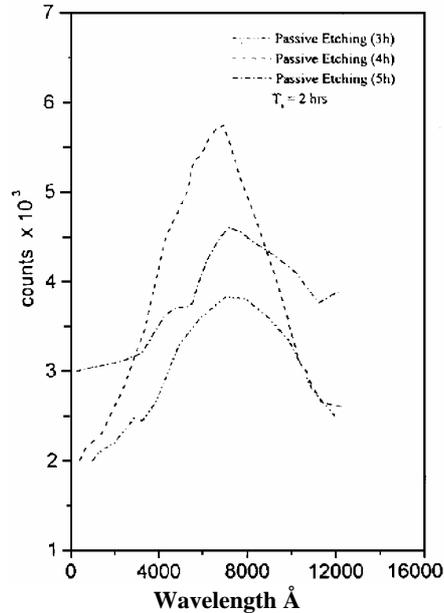
Fig. (1): PL spectra of freshly prepared PSLs and after immersion in ethanol for 2hr then passively etched.
