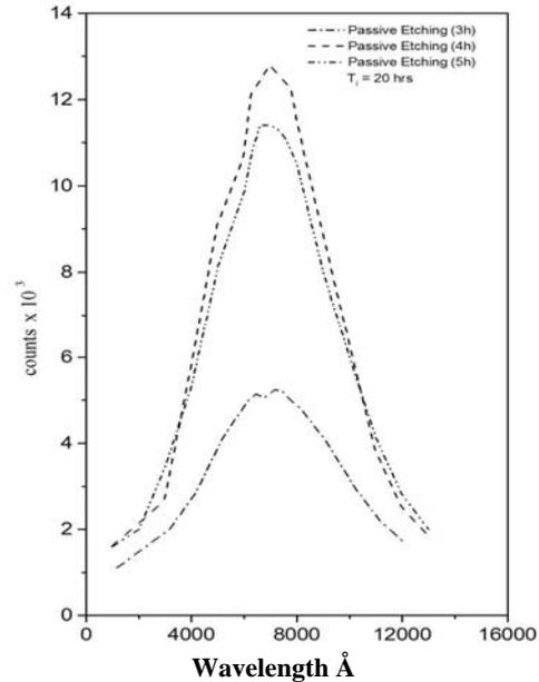
Fig. (2): PL spectra of freshly prepared PSLs and after immersion in ethanol for 20hr then passively etched.
