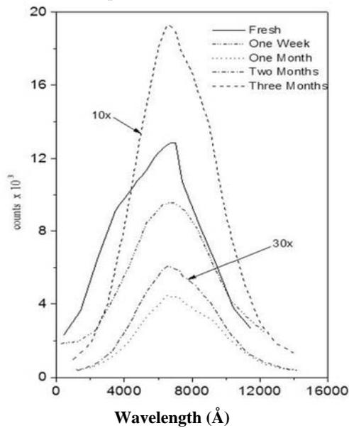
**Fig. (8):** Effect of aging on PL for samples immersed in ethanol for 60hr then passively etched for 2hr and aged up to 3 months.
