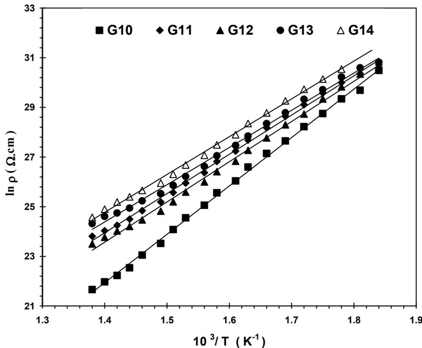
**Fig. (3):** Change of the natural logarithm of electric resistivity  $\ln \rho$  for the investigated glasses versus  $1/T$ .
