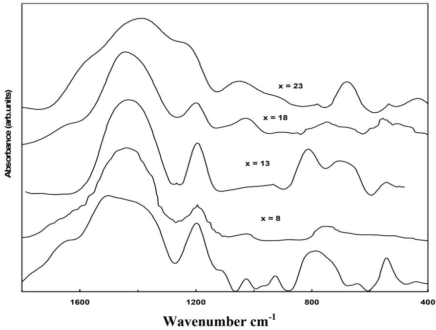
Fig. (1): FTIR absorption spectra for the studied glasses with  $x = 3, 8, 13, 18$  and  $23$  mol % of BaO. Successive spectra have shifted upward.
