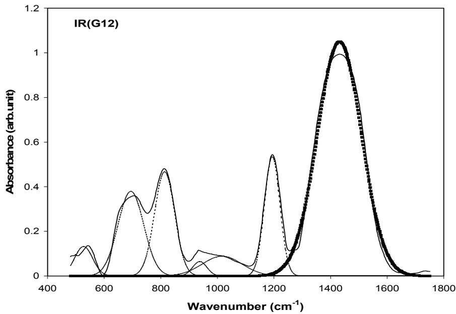
Fig. (2): Deconvolution result for  $13 \text{ BaO} - 3 \text{ Al}_2\text{O}_3 - 78 \text{ B}_2\text{O}_3 - 6 \text{ NaCl}$ , experimental absorption spectrum (solid) and computer bands (dashed lines).
