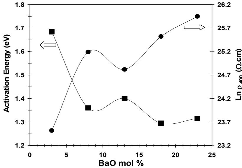
Fig. (4): Change of both the activation energy for the electrical conduction and the natural logarithm of Ln ρ at 400 °C versus the BaO content.
