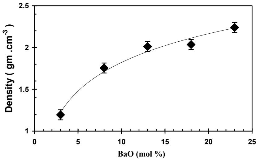
Fig. (5): Change of density with BaO content in the studied glasses. Density data are given in Table (1). The relation between the density (gm / cm<sup>3</sup>) data and BaO content is shown in Fig. (5), where the density
