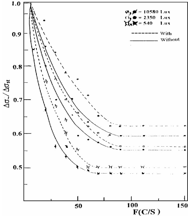
Fig. (3): Relation between the photoconductivity and the chopping frequency at different light intensities with and without side illumination (bias voltage = 30 V).
