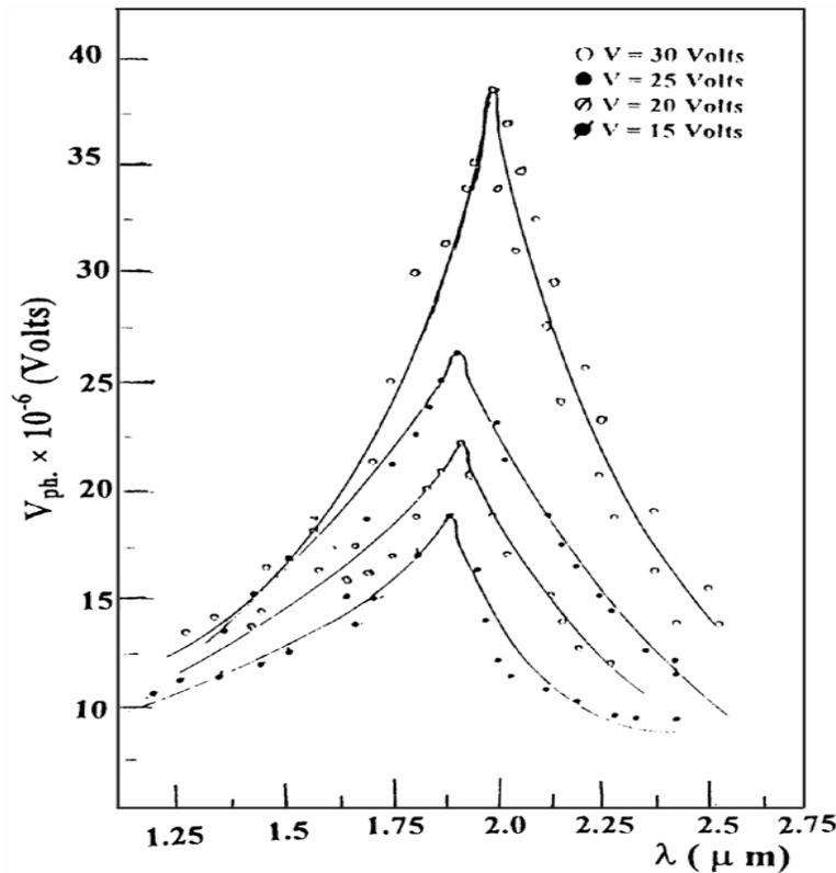
Fig. (1): Variation of the photovoltage with the incident photon wavelengths at different bias voltages.
