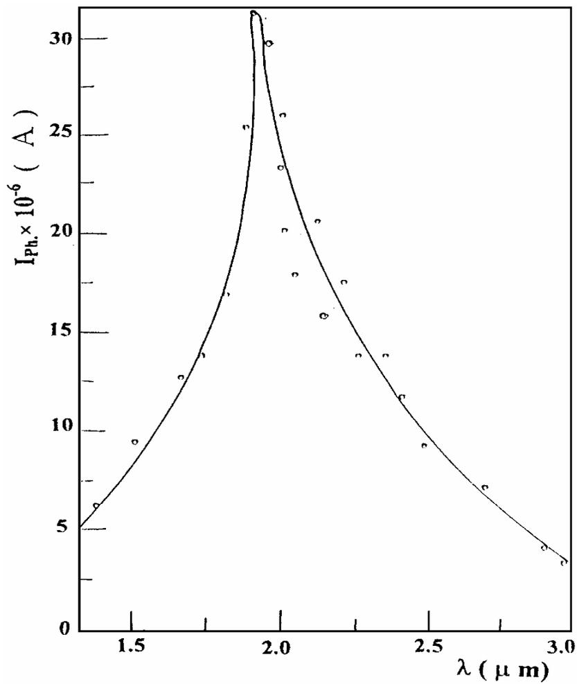
Fig. (6): Spectral distribution of the photocurrent for  $Ga_2Se$  single crystal at bias voltage = 30 V.
