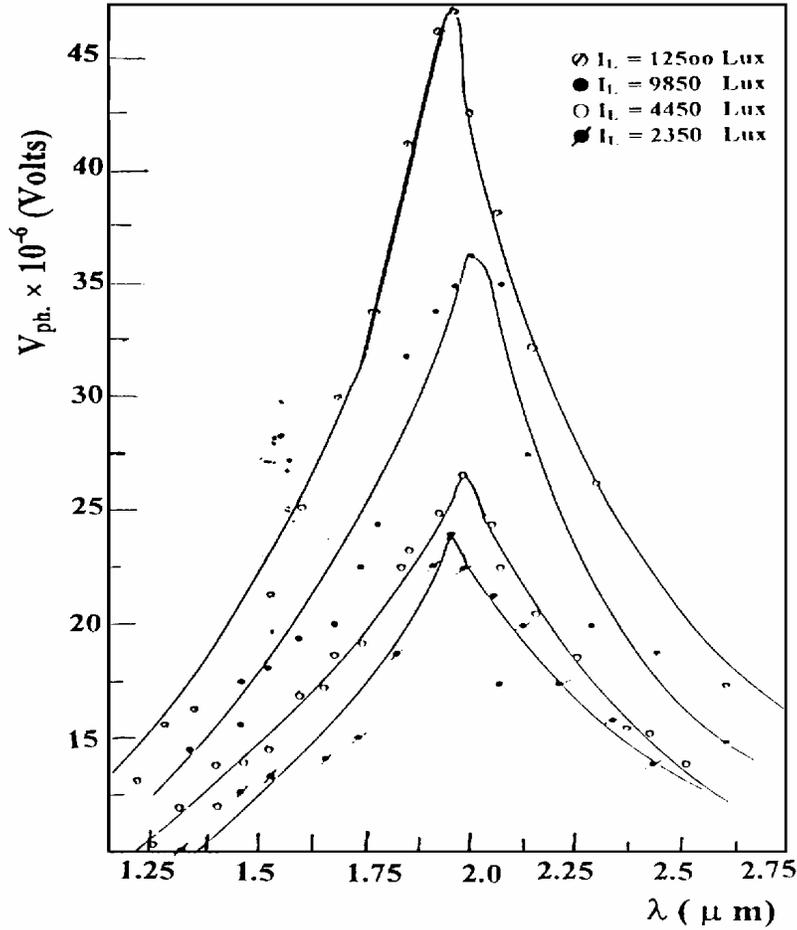
Fig. (2): Variation of the photovoltage with the incident photon wavelengths at different illumination intensities.
