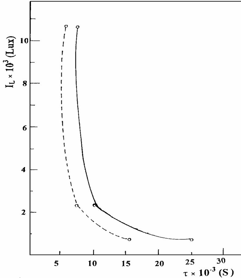
Fig. (4): Dependence of carrier lifetime on light intensity at a bias voltage of 30 (with and without side illumination).
