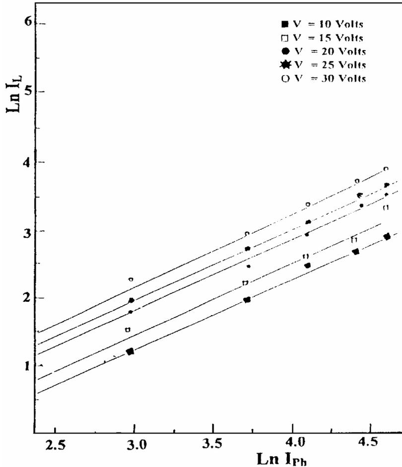
Fig. (5): Dependence of the photocurrent on the light intensity at different bias voltages.
