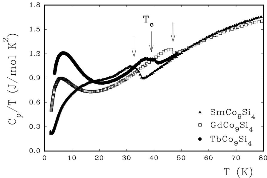
**Fig. (5):** Temperature dependent specific heat  $C_p(T)/T$  versus  $T$  for  $R\text{Co}_9\text{Si}_4$  with  $R = \text{Sm}, \text{Gd}$  and  $\text{Tb}$ .
