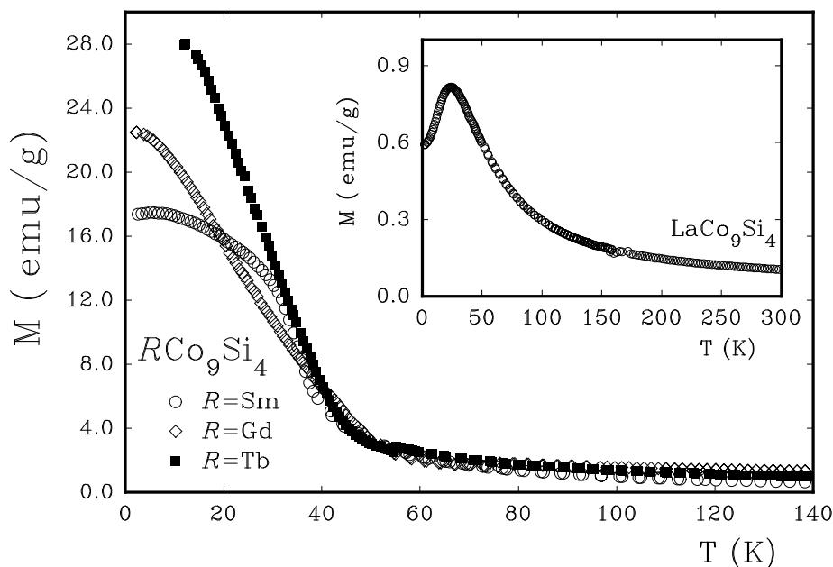
**Fig. (3):** Magnetization versus temperature  $M(T)$  for  $R\text{Co}_9\text{Si}_4$  measured in an applied magnetic field of 1T; the inset shows temperature dependent magnetization measured for  $\text{LaCo}_9\text{Si}_4$ .
