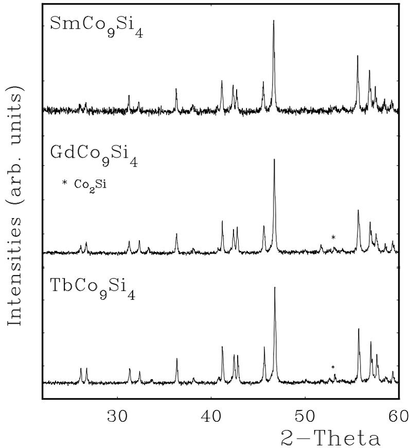
**Fig. (1):** X-ray diffraction patterns of the tetragonal type structure  $RCo_9Si_4$  with  $R =$  Sm, Gd and Tb.
