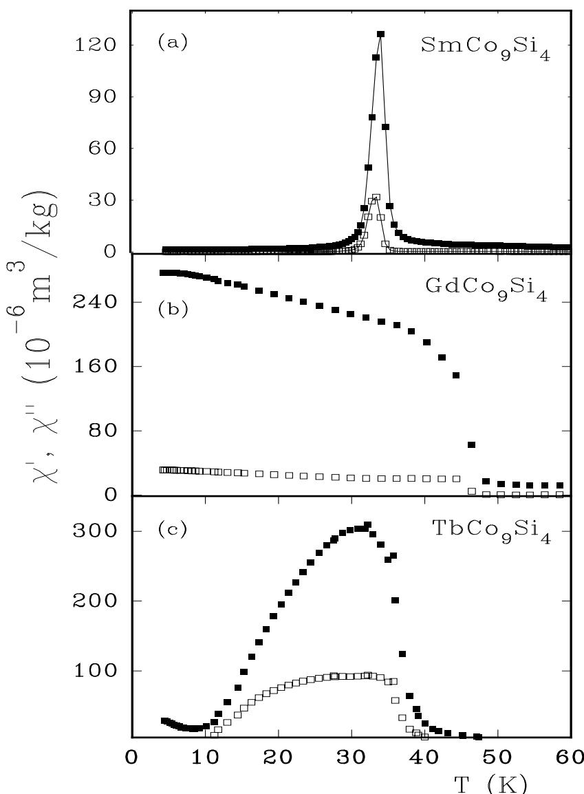
**Fig. (2):** Temperature dependent ac susceptibility  $\chi_{ac}(T)$  of  $R\text{Co}_9\text{Si}_4$  compounds with  $R = \text{Sm}$ ,  $\text{Gd}$  and  $\text{Tb}$ . Full symbols are the real part ( $\chi'$ ) of the ac susceptibility while the open symbols represent the imaginary part ( $\chi''$ ).
