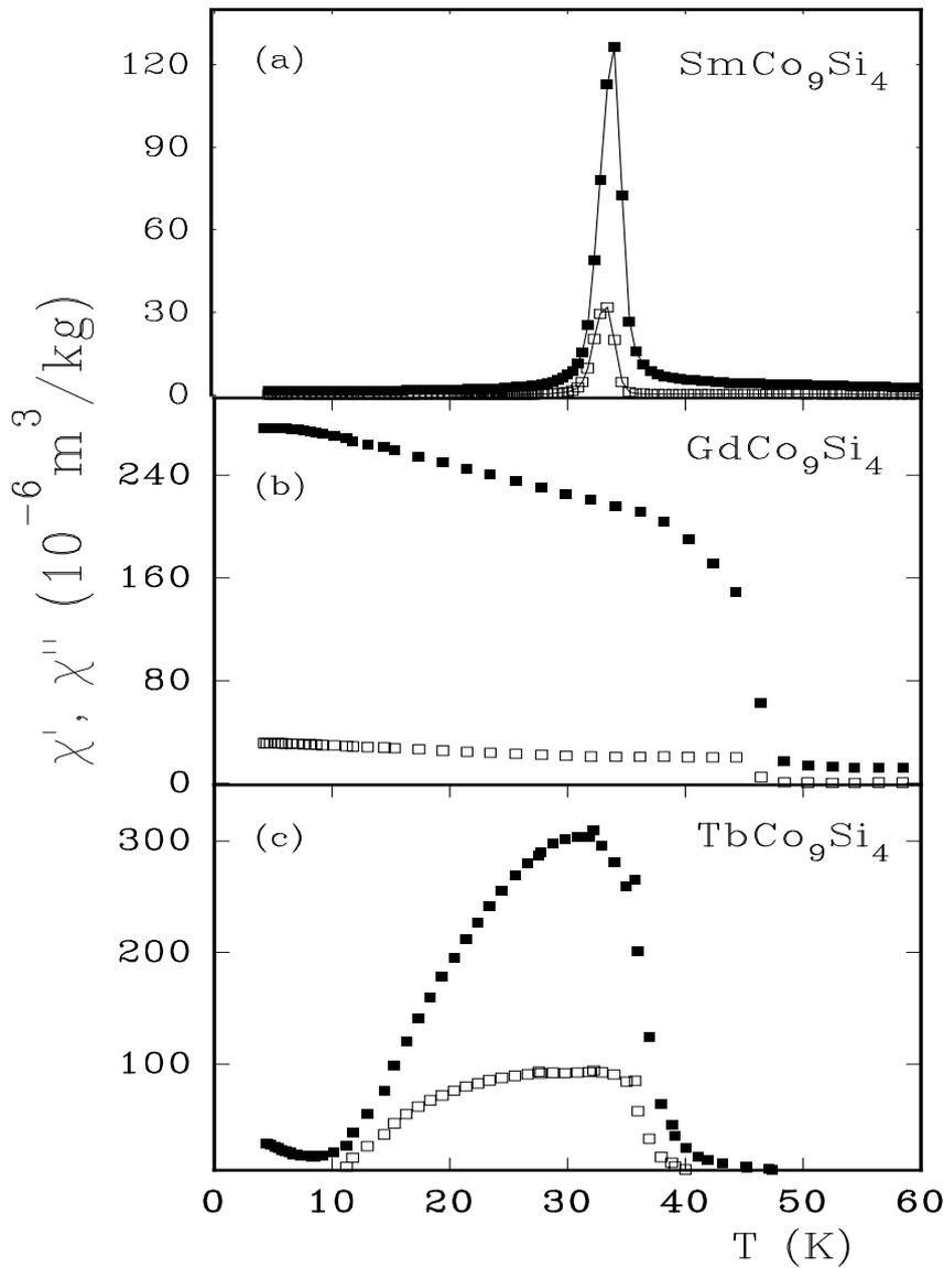
**Fig. (2):** Temperature dependent ac susceptibility  $\chi_{ac}(T)$  of  $RCo_9Si_4$  compounds with  $R = Sm, Gd$  and  $Tb$ . Full symbols are the real part ( $\chi'$ ) of the ac susceptibility while the open symbols represent the imaginary part ( $\chi''$ ).
