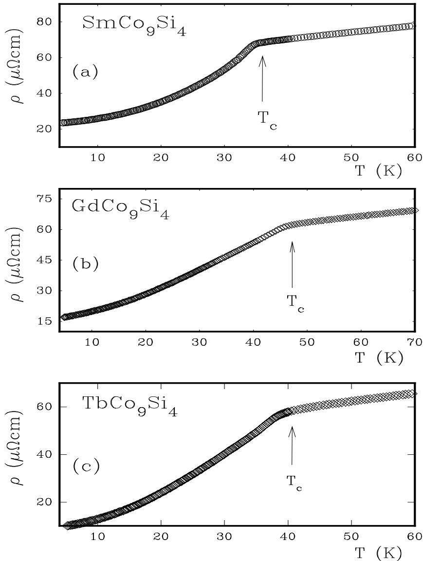
**Fig. (4):** Temperature dependent electrical resistivities  $\rho(T)$  for  $R\text{Co}_9\text{Si}_4$  with (a)  $R = \text{Sm}$ , (b)  $R = \text{Gd}$ , and (c)  $R = \text{Tb}$ .
