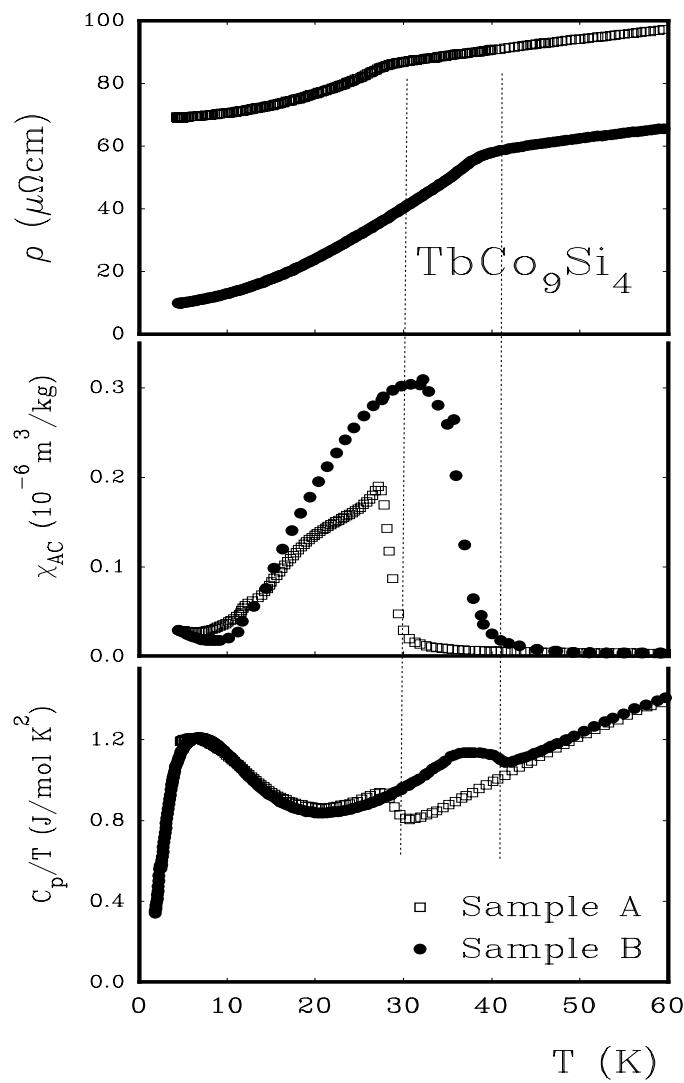
**Fig. (6):** Temperature dependent resistivity, susceptibility, and specific heat measurements of two  $\text{TbCo}_9\text{Si}_4$  samples A and B.
