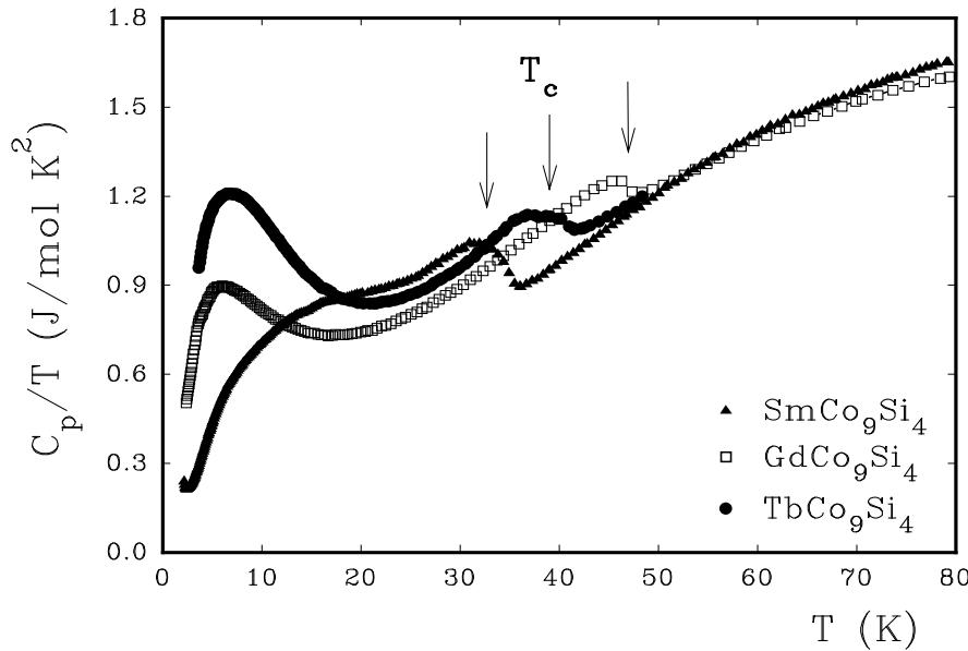
**Fig. (5):** Temperature dependent specific heat  $C_p(T)/T$  versus  $T$  for  $R\text{Co}_9\text{Si}_4$  with  $R = \text{Sm, Gd and Tb}$ .
