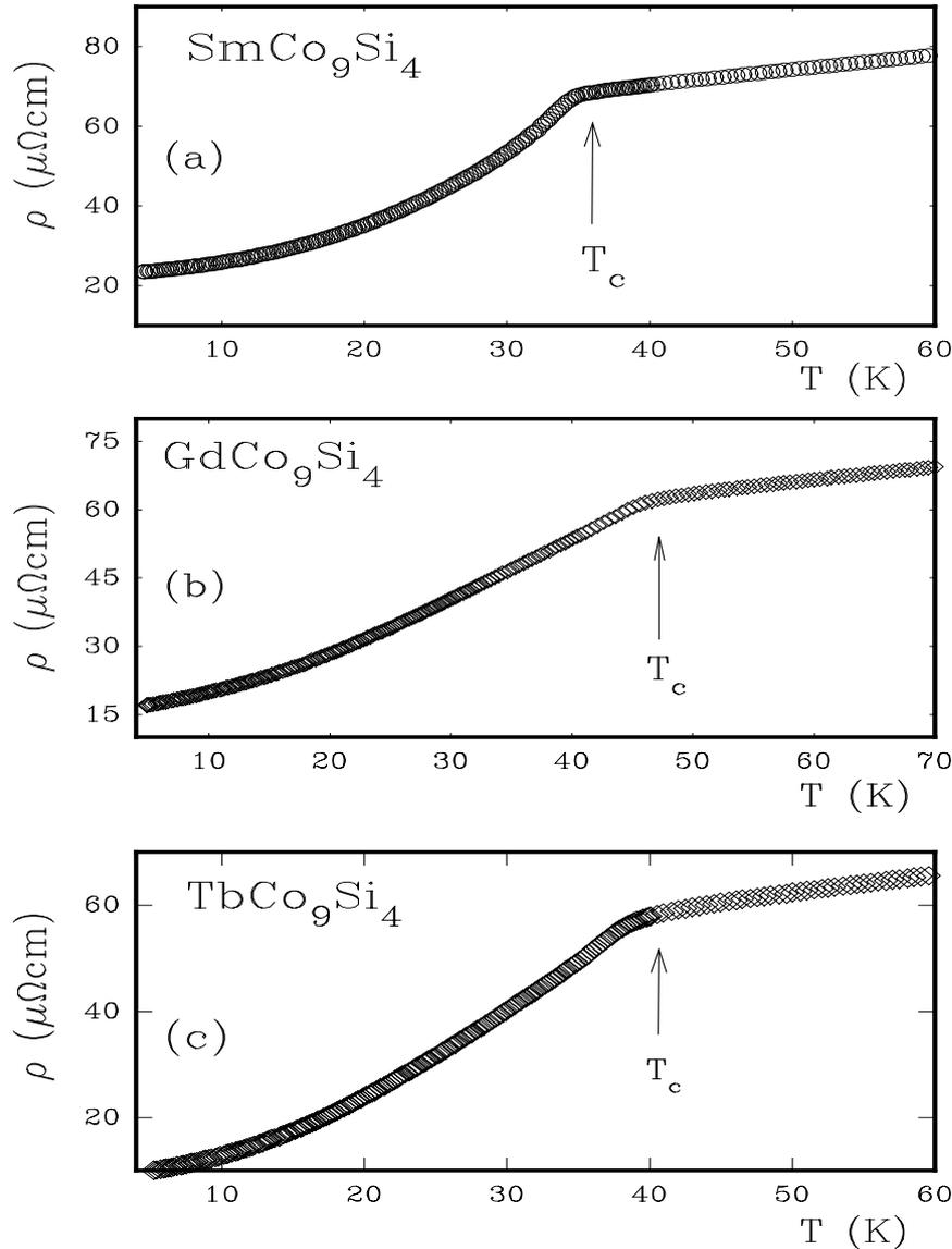
**Fig. (4):** Temperature dependent electrical resistivities  $\rho(T)$  for  $R\text{Co}_9\text{Si}_4$  with (a)  $R = \text{Sm}$ , (b)  $R = \text{Gd}$ , and (c)  $R = \text{Tb}$ .
