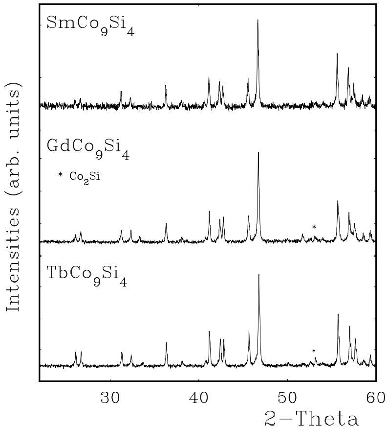
**Fig. (1):** X-ray diffraction patterns of the tetragonal type structure  $R\text{Co}_9\text{Si}_4$  with  $R = \text{Sm, Gd and Tb}$ .
