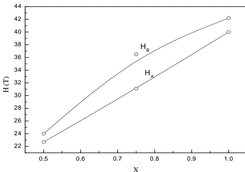
**Fig. (5):** The variation of the hyperfine magnetic fields  $H_A$  and  $H_B$  (for A- and B- site respectively) with  $Mn^{2+}$  ions content.
