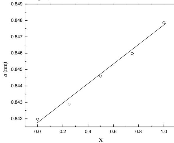
**Fig. (2):** The variation of the lattice constant,  $a$ , with  $\text{Mn}^{2+}$  ions content.
