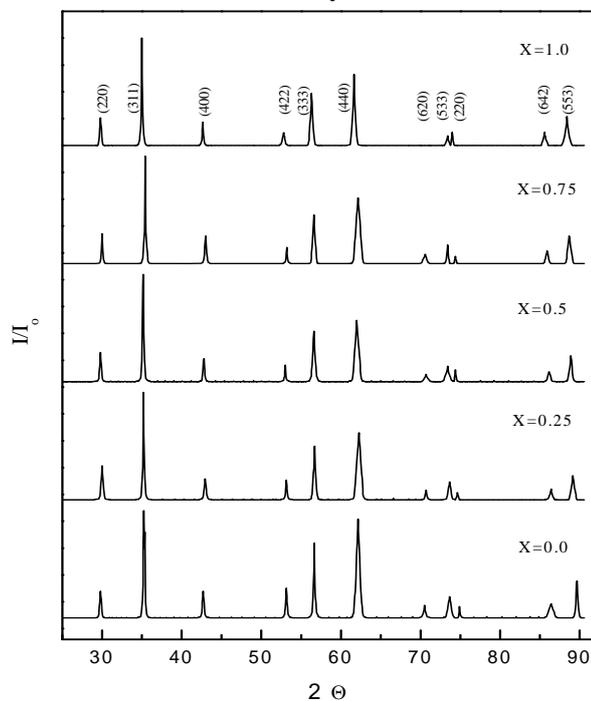
**Fig. (1):** X-ray diffraction pattern for  $\text{Mn}_x\text{Zn}_{1-x}\text{Fe}_2\text{O}_4$  system.
