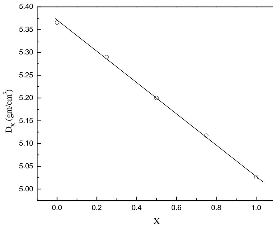
**Fig. (3):** The variation of the X-ray density with Mn<sup>2+</sup> ions content.
