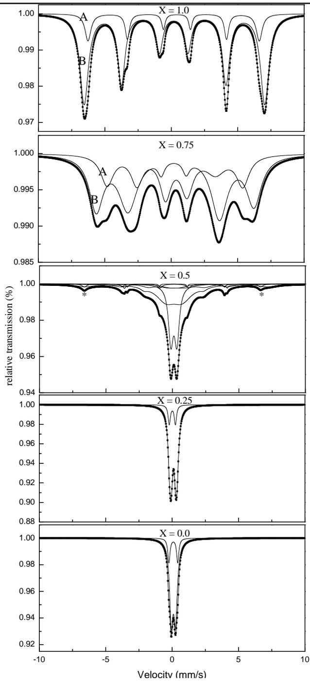
**Fig. (4):** Room temperature Mössbauer spectra of  $\text{Mn}_x\text{Zn}_{1-x}\text{Fe}_2\text{O}_4$  system.
